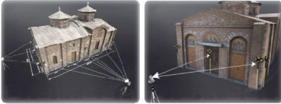
Figure 6. Representation of the photogrammetric method
